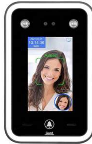
LED Frame plastic case Bell button 4.3 Inch IPS Touch Screen
